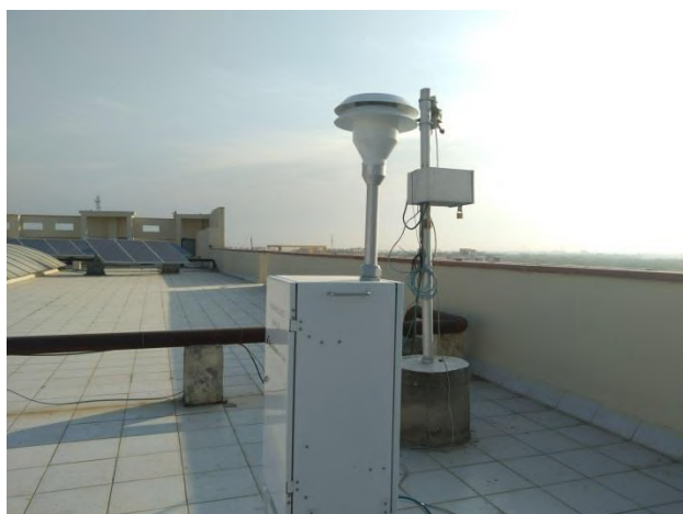
PM Sampler installed under UGC-BSR Startup Grant on
