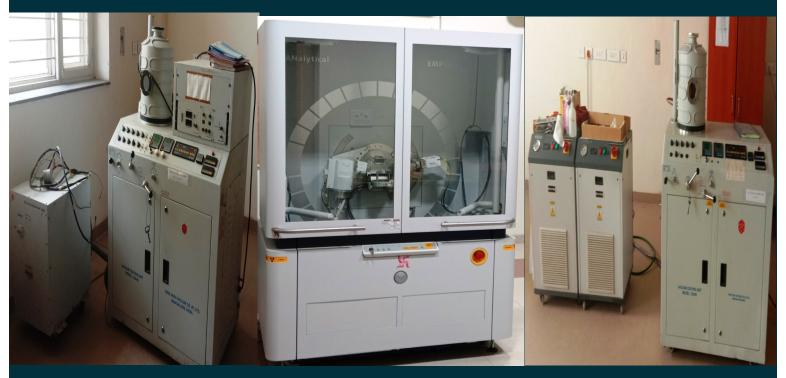
E-Beam Vacuum Coating Unit **XRD**
